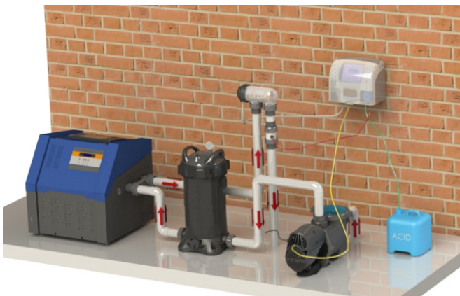
Figure 2. Equipment Configuration, Acid Dosing
